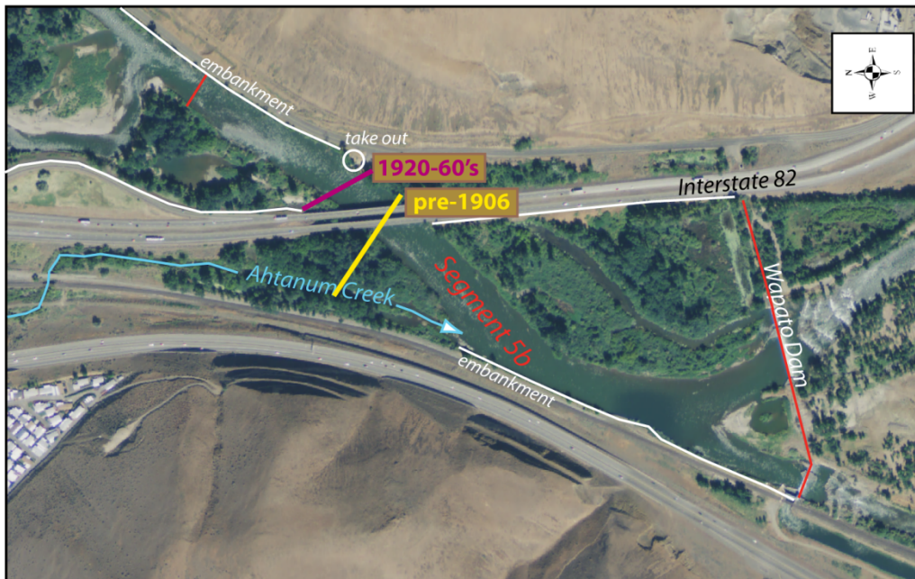
Figure 13: Segment 5b location map, 2009 aerial photography. Purple and yellow lines indicate approximate locations of previous bridges over the Yakima River. White lines indicate embankments. Flow is from left to right
