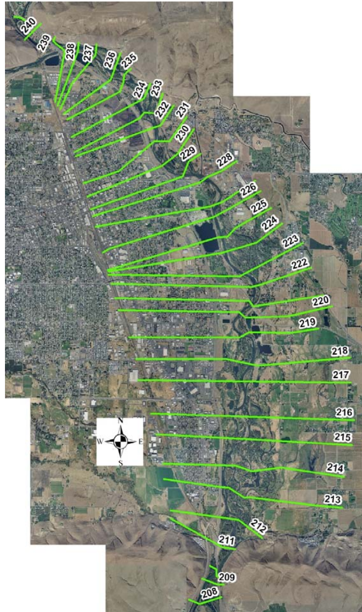
Figure 27: 1969 cross section alignments overlaid on aerial photography (2005). These alignments were provided by Yakima County and used to determine 2005 elevations for comparison.
