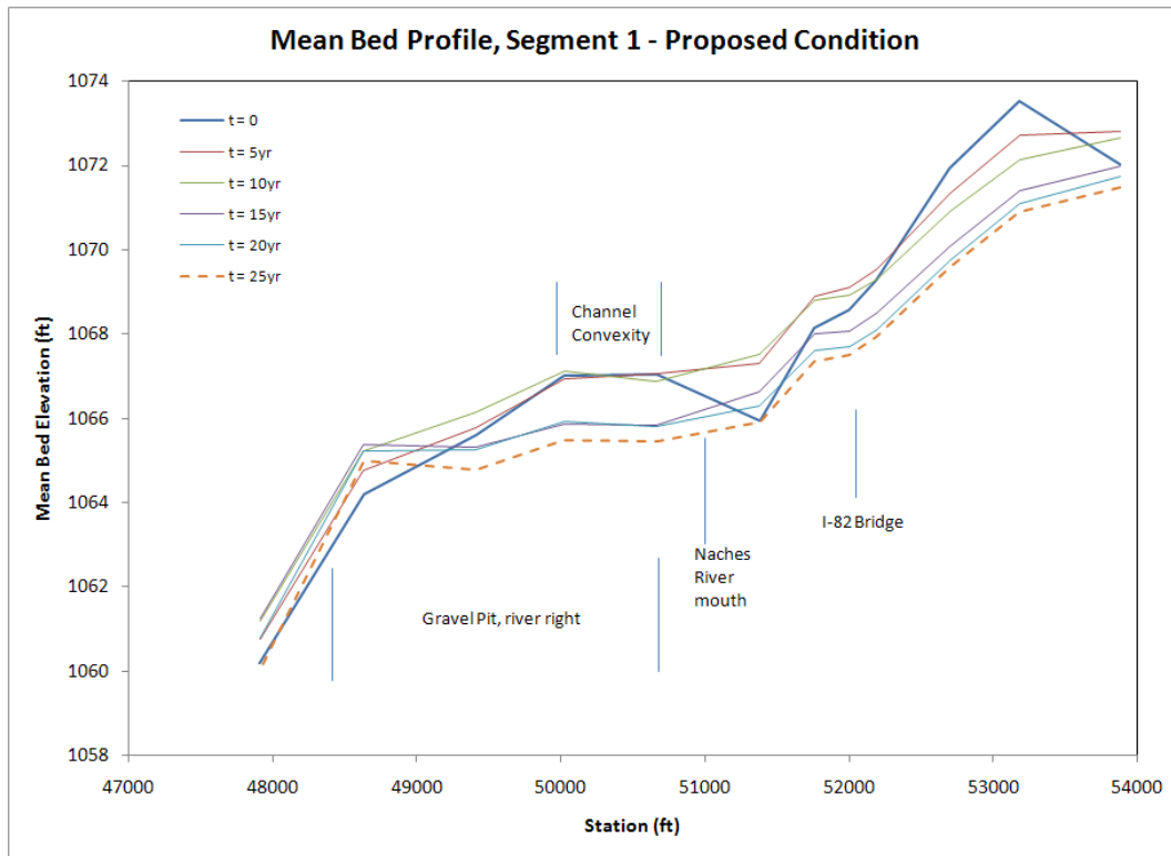
Figure 71: Profile of mean bed elevations in segment 1 throughout the modeling period.
