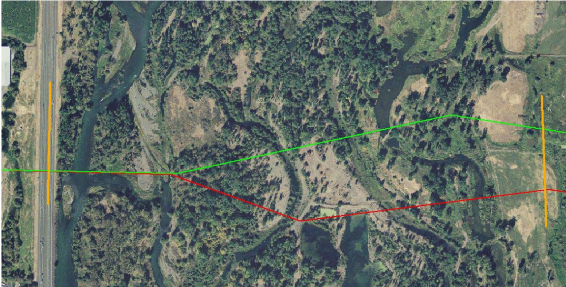
Figure 7 – Alignment of cross section 214 overlain on 2005 photo. Green line is alignment from Corps Study, red line is new alignment based on fitting the cross section plot to topography.
