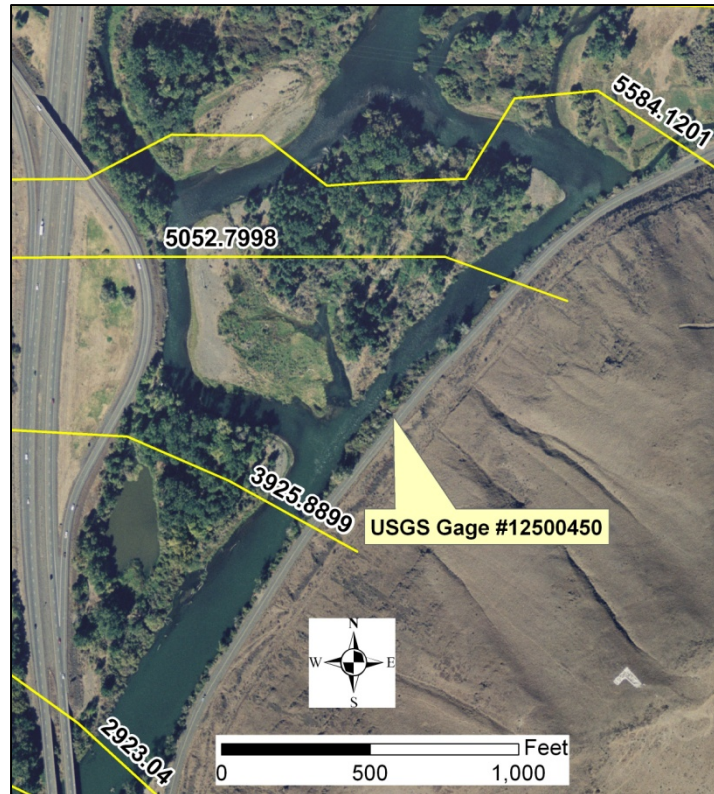
Figure 58: Photograph showing the location of cross section 5052.8, the upstream extent of the influence of Wapato Dam.
