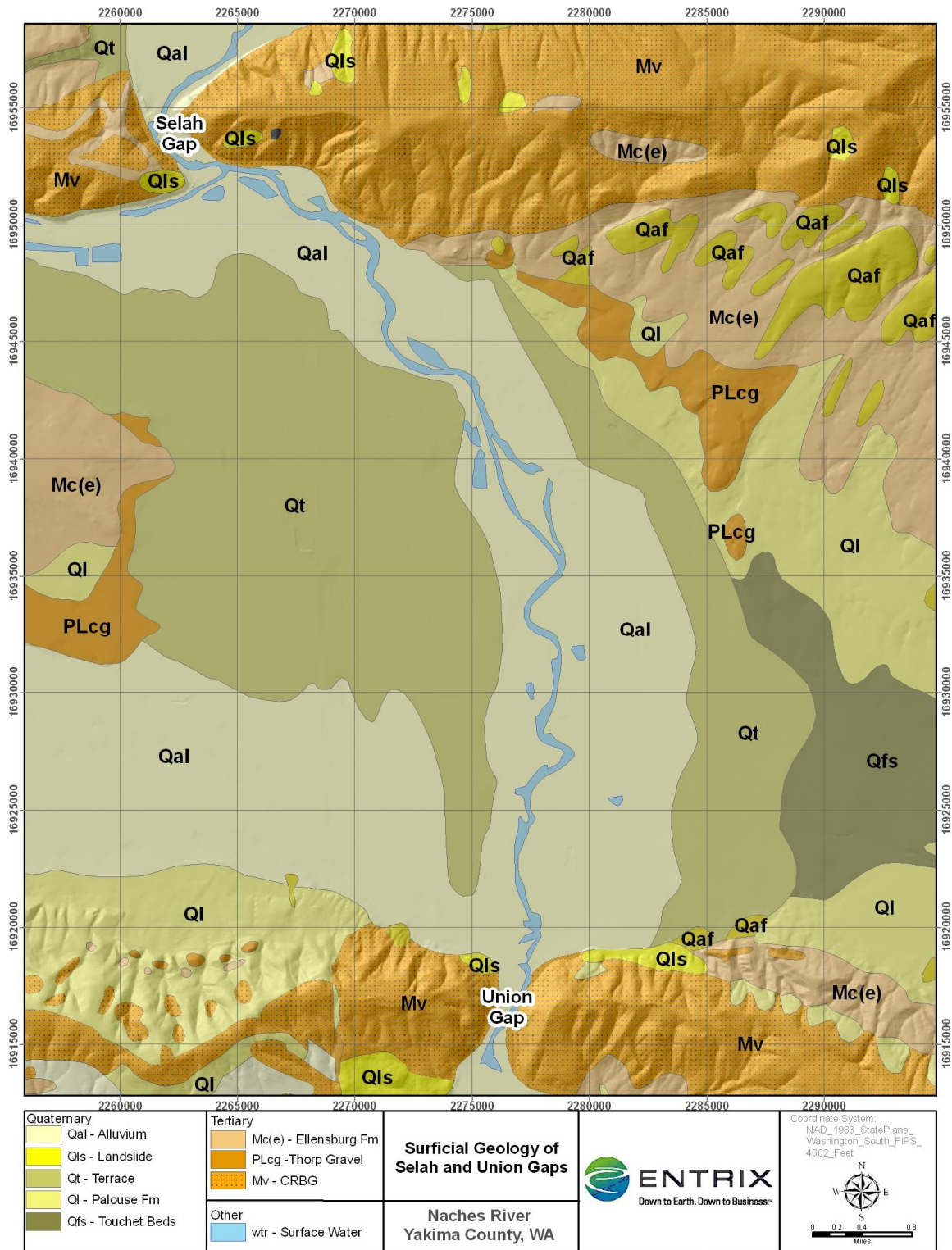
Figure 16 Surface Geology of the Selah to Union Gap Reach on the Yakima River. Note the outcrops of the CRBG (Mv) on both the east and west valley walls at the gaps. Geology data provided by Yakima County.
