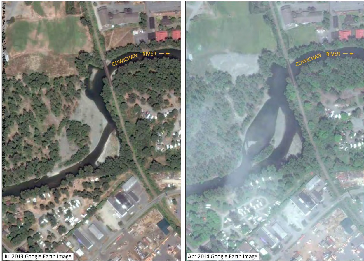
Figure 38: Example of a chute cutoff side channel development at a bend
