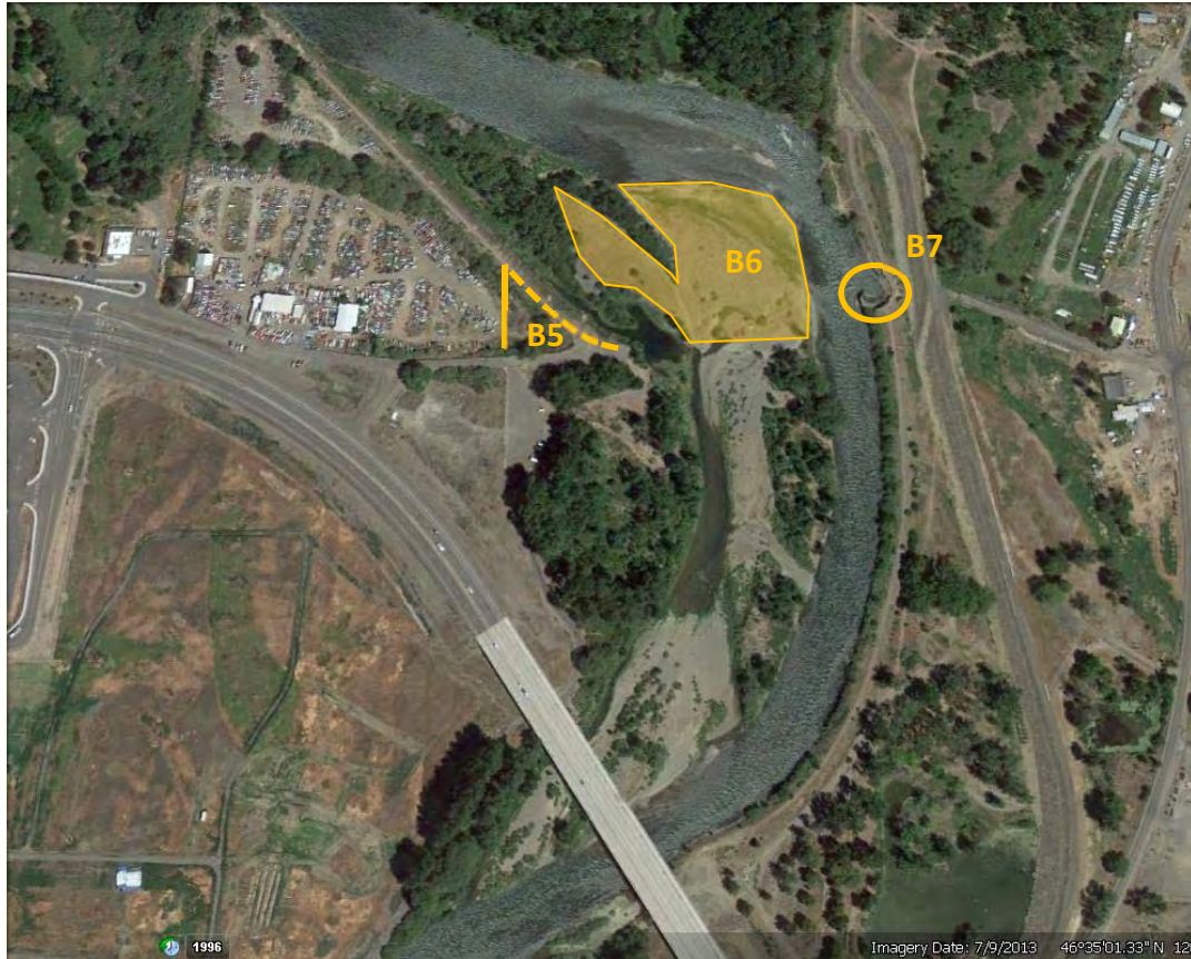
Figure 44: Alternatives (B5) Removal of Nob Hill levee segment, (B6) gravel bar excavation on west bank point bar, and (B7) removal of old SR24 abutment.
