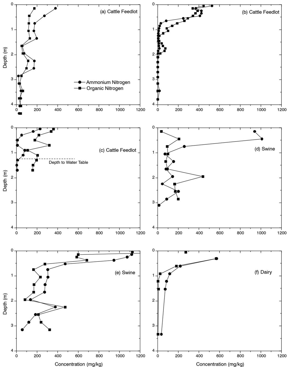
Figure 5. Profiles of ammonium nitrogen and organic nitrogen beneath six older lagoons.
