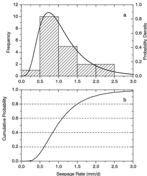
Figure 2. Histogram of the whole-lagoon seepage rates measured from 20 lagoons (table 1). Also shown are (a) the probability density curve and (b) the cumulative probability curve for the lognormal distribution as calculated from the mean and variance of the seepage data.
