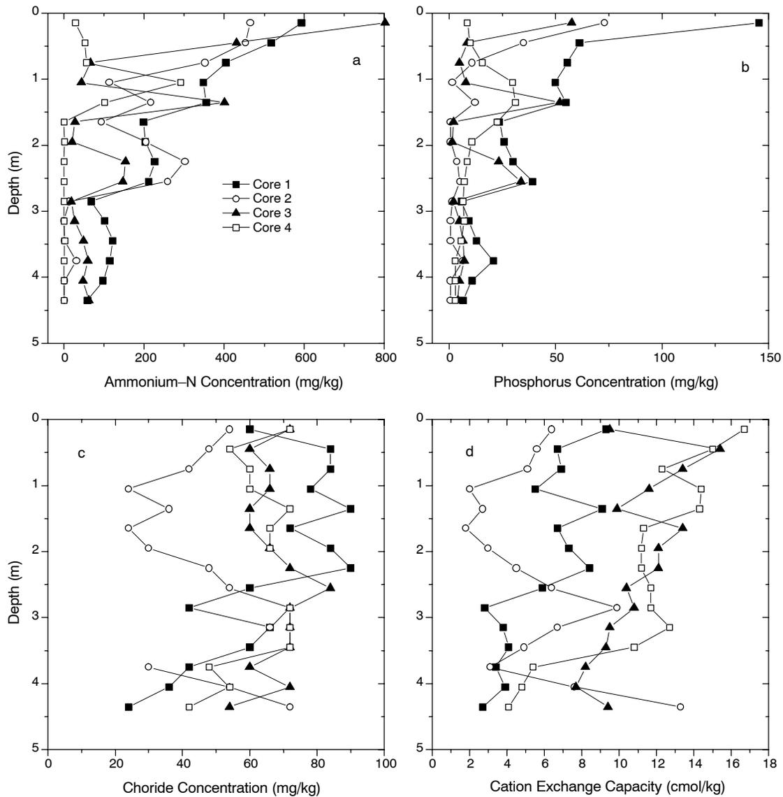
Figure 6. Profiles of (a) ammonium nitrogen, (b) phosphorus (Olsen-P), (c) chloride, and (d) cation exchange capacity at four different locations in the bottom of the 2.8-ha, 11-year-old cattle feedlot lagoon (same location as fig. 5a). Cores were collect along a transect at 30-m intervals.
