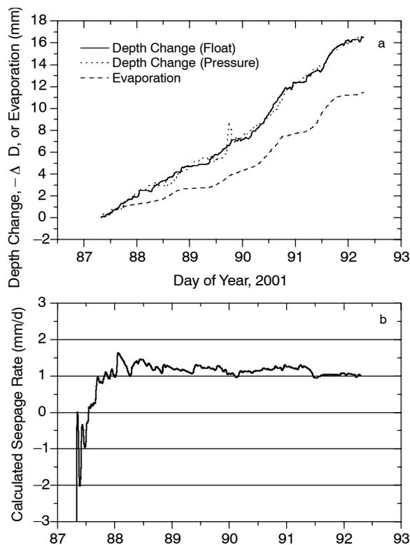
Figure 1. Results from a five-day water balance test at a cattle feedlot lagoon. Included are (a) cumulative change in depth and evaporation, and (b) the apparent seepage rate as calculated at different times following the start of the test. Changes in depth were measured with float- and pressure-based recorders.
