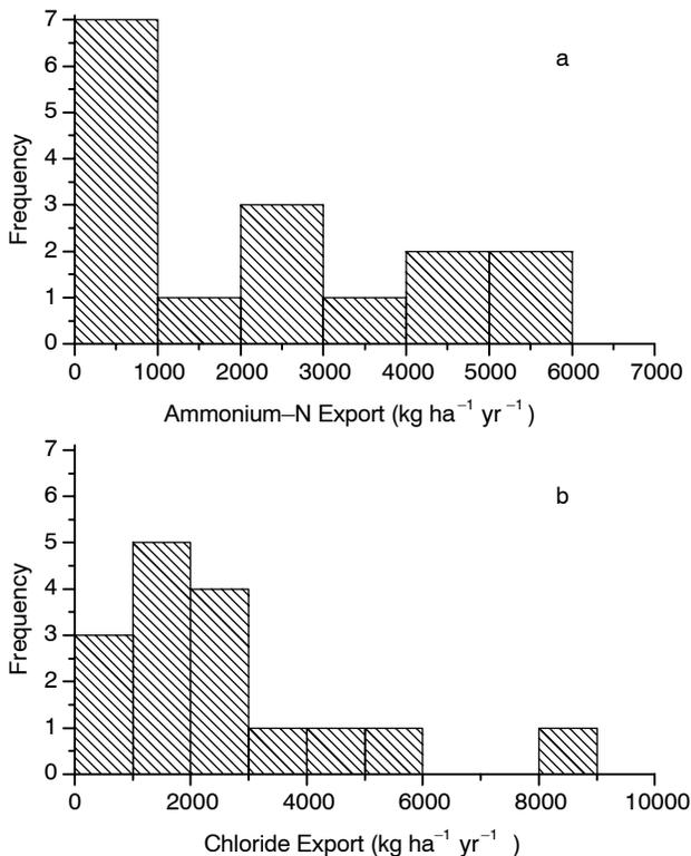
**Figure 4.** Annual subsurface export rates of (a) ammonium-N and (b) chloride from the 20 lagoons listed in table 1. Data were calculated from the seepage rate and the corresponding chemical concentration of  $\text{NH}_4^+$ -N and  $\text{Cl}^-$  in each lagoon.
